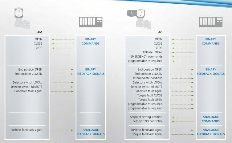
Cost reduction is one of the main factors in favour of fieldbus technology. In addition, introduction of serial communication in process automation has proven as an innovation driver for field devices and consequently for actuators. Concepts for efficiency gains such as remote parameterisation or Plant Asset Management would not be feasible without fieldbus technology. AUMA actuators equipped with fieldbus interfaces are state of the art.
