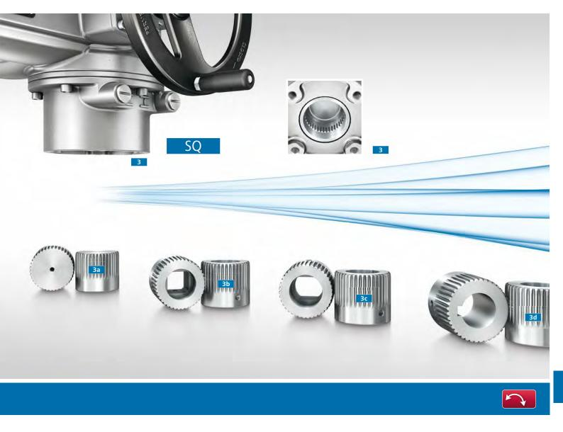
For part-turn actuators, connection to the valve has to comply with EN ISO 5211. Like for the output drive plug sleeve for SA multi-turn actuators, SQ actuators provide a splined coupling for torque transmission.
